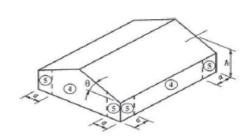
The width of zone 5 is the 'a' distance; it is either 10% of the least horizontal dimension of the structure - or - 0.4 times the mean roof height, but not less than 4% of the least horizontal distance -or- 3 feet. It is measured from the corner of the structure. Note that 3-feet is not the default value, it is the minimum width.
